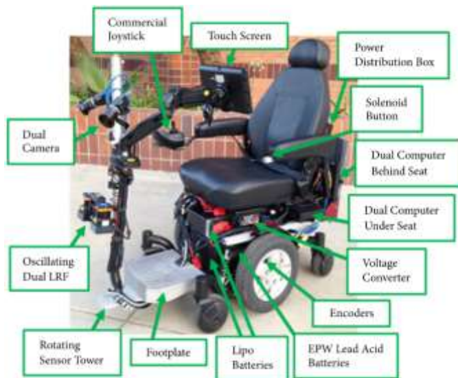
Fig. 1 A basic smart wheelchair system without proposed modules[16-17]
